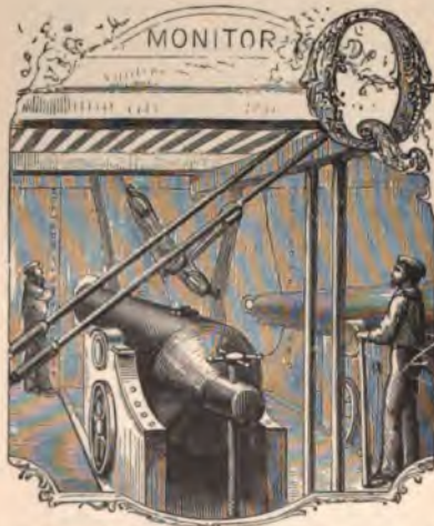
INTERIOR OF THE TOWER OF THE MONITOR.
